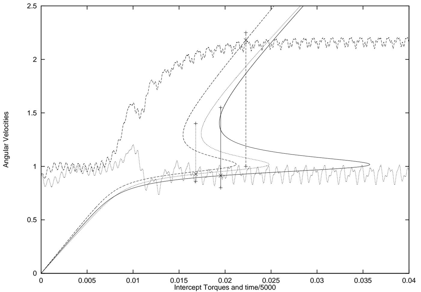
Figure 7. INDIVIDUAL CRANK SPEEDS VS. TIME AND THREE RESONANCE CURVES — SHAKERS DO NOT LOCK IN — Parameter Values:  $c_{av} = 0.2$ ,  $(m_{ecc}e)_{av} = 0.1$ ,  $D_{av} = 0.01$ ,  $J_{av} = 0.2$ ,  $(T_{intercept})_{av} = 0.01952$ ,  $r_M = -1/20$ ,  $r_D = -1/20$ ,  $r_J = -1/20$ ,  $r_T = +0.14$ .
