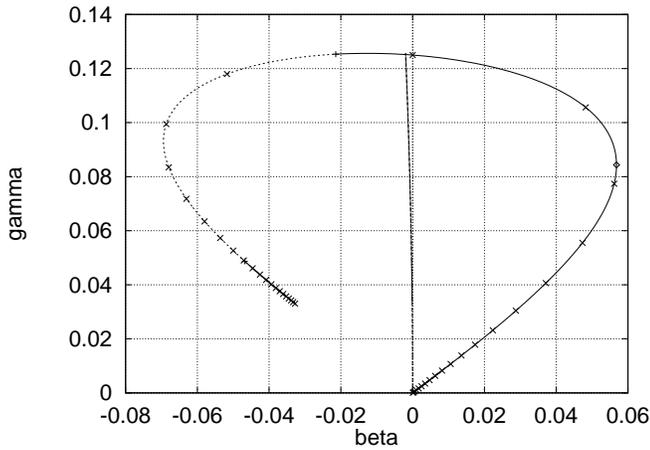
Figure 2. 'RESONANCE CURVE' IN  $\beta, \gamma$  COORDINATES AND LOW  $\beta$  STABILITY BOUNDARY — Parameter Values:  $c_{av} = 0.2$ ,  $(m_{ecc}e)_{av} = 0.1$ ,  $D_{av} = 0.01$ ,  $J_{av} = 0.2$  ( $m_{av} = 1$ ,  $k_{av} = 1$ , and  $e_{av} = 1$ ).
