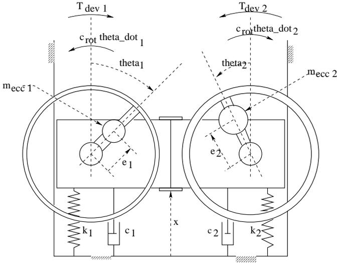
Figure 1. COMMON BASE COUPLED, TWO ECCENTRIC DRIVEN, NONLINEAR OSCILLATING SYSTEM
