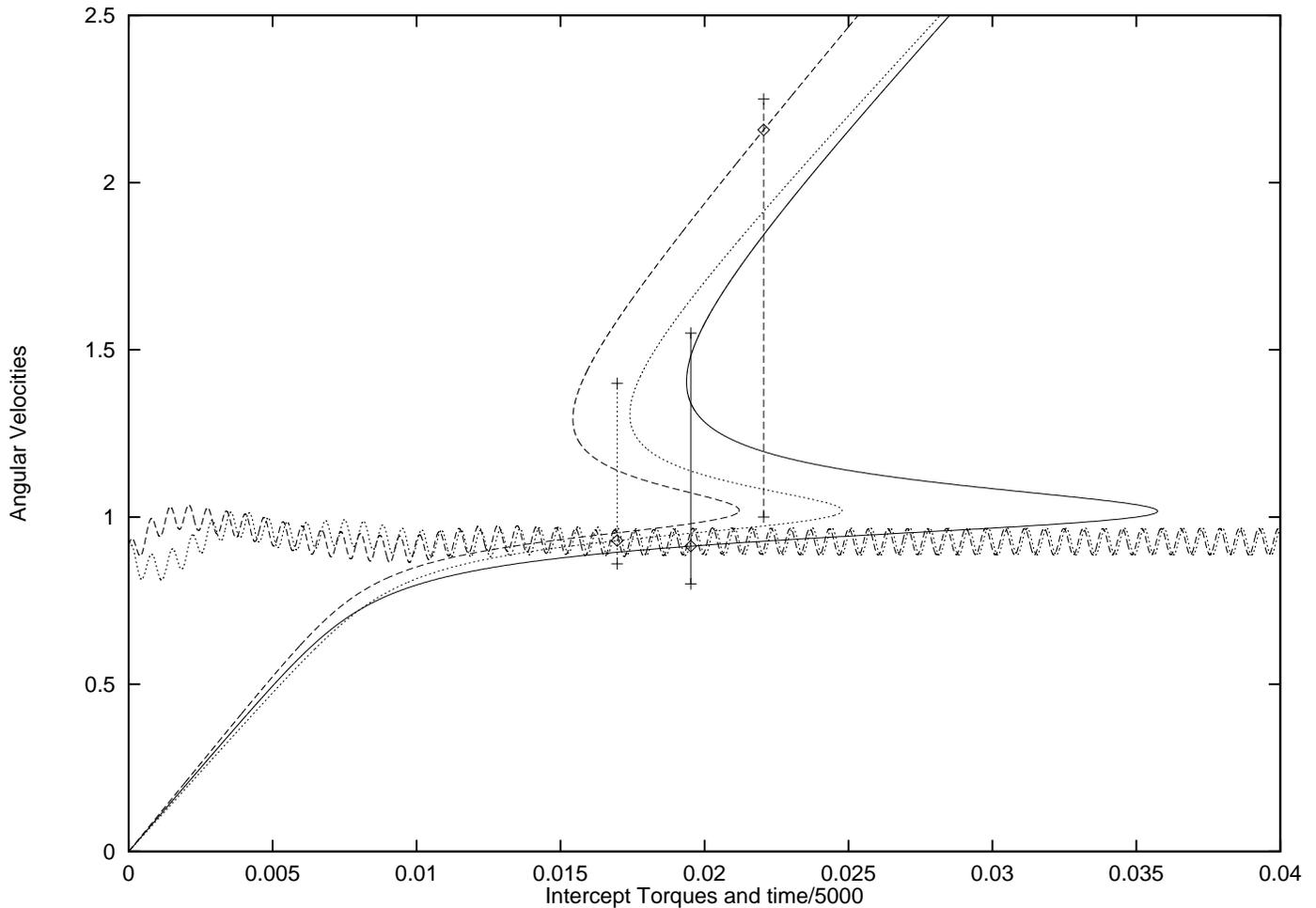
Figure 6. INDIVIDUAL CRANK SPEEDS VS. TIME AND THREE RESONANCE CURVES —SHAKERS LOCK IN — Parameter Values:  $c_{av} = 0.2$ ,  $(m_{ecc}e)_{av} = 0.1$ ,  $D_{av} = 0.01$ ,  $J_{av} = 0.2$ ,  $(T_{intercept})_{av} = 0.01952$ ,  $r_M = -1/20$ ,  $r_D = -1/20$ ,  $r_J = -1/20$ ,  $r_T = +0.13$ .
