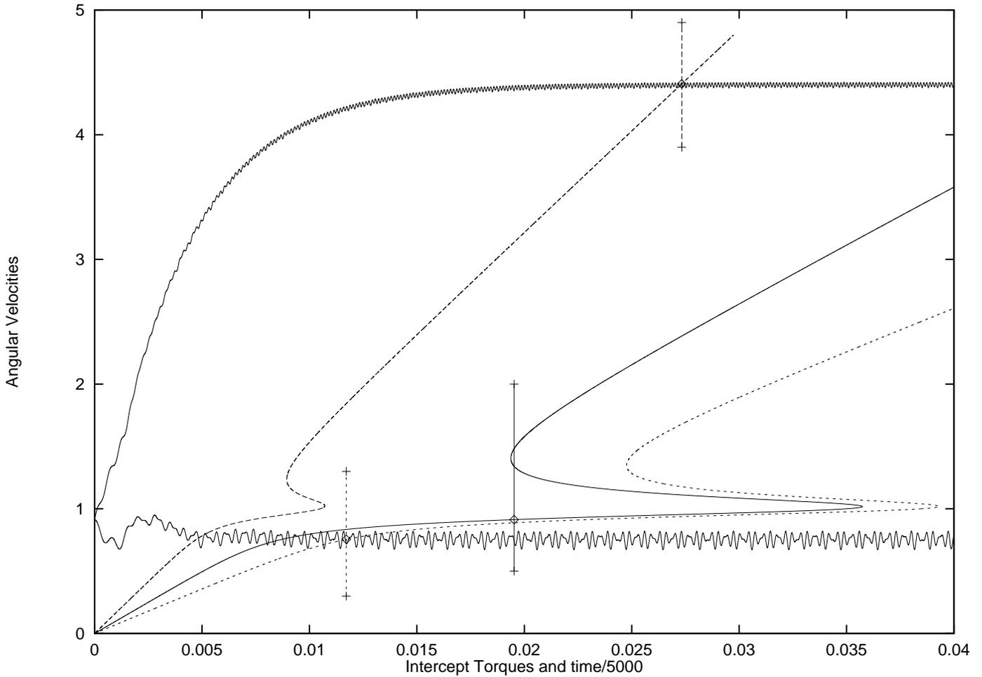
Figure 5. INDIVIDUAL CRANK SPEEDS VS. TIME AND THREE RESONANCE CURVES — SHAKERS DO NOT LOCK IN — Parameter Values:  $c_{av} = 0.2$ ,  $(m_{ecc}e)_{av} = 0.1$ ,  $D_{av} = 0.01$ ,  $J_{av} = 0.2$ ,  $(T_{intercept})_{av} = 0.01952$ ,  $r_M = 8 \cdot (-1/20)$ ,  $r_D = 8 \cdot (-1/20)$ ,  $r_J = 8 \cdot (-1/20)$ ,  $r_T = 8 \cdot (+1/20)$
